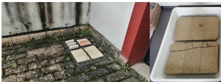
Location of the specimens in a humid area on a terrace of the IAPH headquarters during the first 6 months (left) and in trays in the laboratory for the remainder of the test (right).
