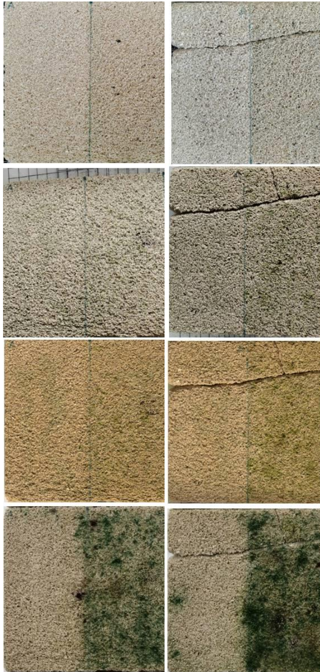
Evolution of the Puerto stone specimens during the test. From top to bottom, at 3, 6, 9 and 12 months. In all cases, on the left the area treated with Aquashield Active and on the right the untreated area.
