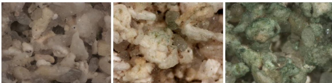
Stereomicroscope images (7x) of uncolonised Puerto stone (left), incipient colonisation in area treated with Aquashield Active (centre) and full colonisation in untreated area (right). Regardless of whether they are treated or untreated, the photosynthetic microorganisms present have the same vitality.
