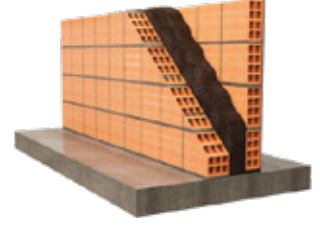
Internal partitions Filling the internal double walls with expanded cork granules
