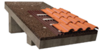
Roofs Pitched roof with corrugated roofing system
