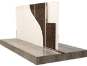
Internal partitions Metal-stud wall and slab discontinuity
