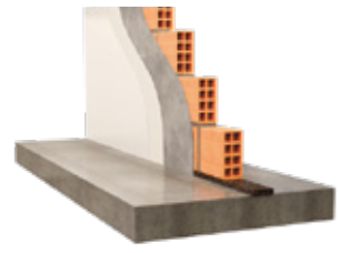
Internal partitions Masonry wall and slab discontinuity
